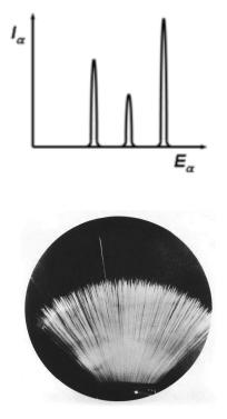
Figure 3. A discrete energy spectrum of alpha radiation.
