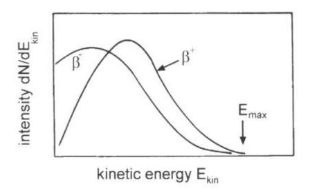
Figure 2. A continuous energy spectrum of beta radiation.
